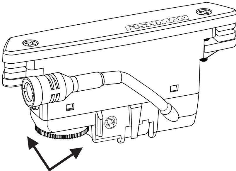
Rotate thumbwheel counterclockwise for full pickup
